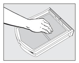
Use your fingers or a vacuum cleaner to remove the fluff from the surface of the filter.
